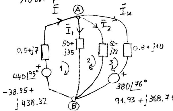
$$\begin{bmatrix} 1 & -1 & -1 & -1 \\ 0.5+j7 & 50+j35 & 0 & 0 \\ 0 & -50 & 60-j22 & 0 \\ 0 & 0 & 0.8 & +j10 \end{bmatrix} \begin{bmatrix} \bar{I} \\ \bar{I}_1 \\ \bar{I}_2 \\ \bar{I}_K \end{bmatrix} = \begin{bmatrix} 0 \\ -3835+j438.32 \\ 0 \\ -91.93-j368.71 \end{bmatrix}$$
