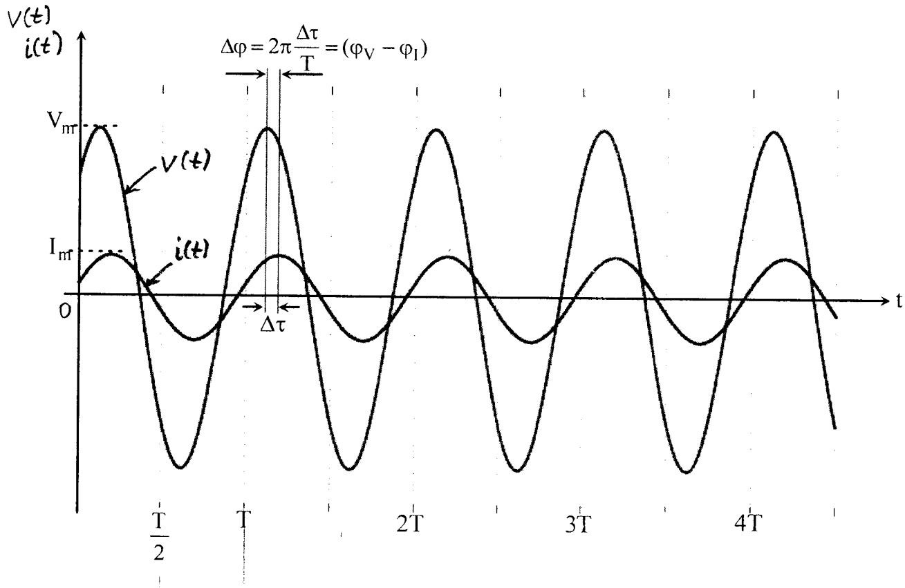
$$p(t) = \frac{1}{2} V_m I_m \cos(\varphi_V - \varphi_I) - \frac{1}{2} V_m I_m \cos(2\omega t + \varphi_V + \varphi_I)$$
