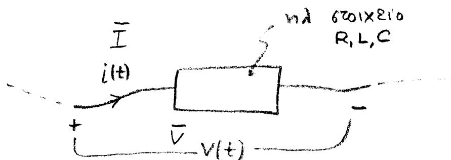
$$V(t) = V_m \sin(\omega t + \varphi_V) \rightarrow \bar{V} = V_m e^{j\varphi_V}$$
