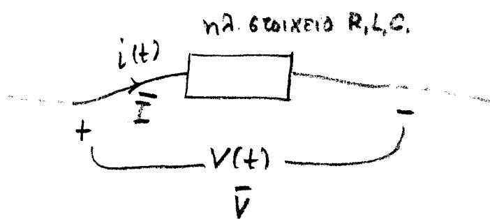
$$V(t) = V_m \sin(\omega t + \varphi_V) \rightarrow \bar{V} = V_m e^{j\varphi_V}$$
