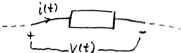
$$V(t) = 120 \sin(\omega t + 12^\circ) \text{ V}, \quad i(t) = 4 \sin(\omega t - 40^\circ) \text{ A}$$
